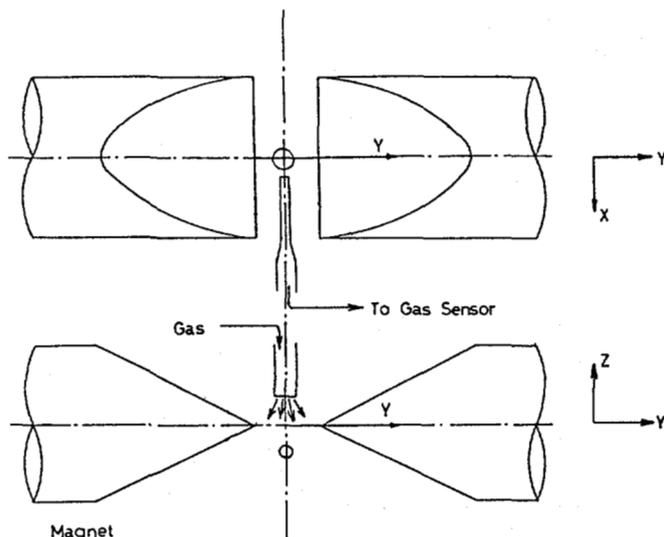
Fig. 3 Experimental setup to observe gas flow under magnetic fields.
