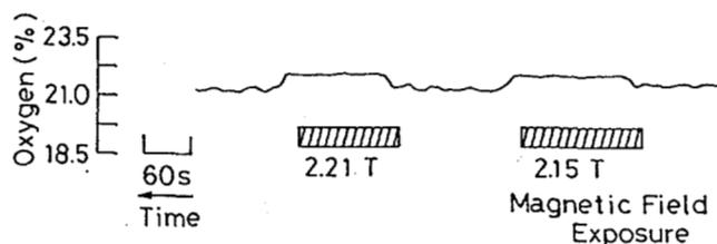
Fig. 5 Gas-flow changes during magnetic field exposures when oxygen gas is supplied.
