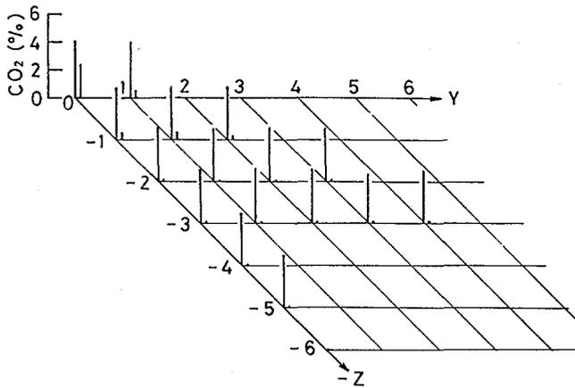
Fig.6 Spatial distributions of carbon dioxide in the lower half plane of the airgap when carbon dioxide is supplied at  $z=8.0$  mm. A column in the left side at each lattice point shows carbon-dioxide concentration before magnetic field exposures and a column in the right side shows carbon-dioxide concentration during magnetic field exposures. Gas flow is blocked by the magnetic fields. The field intensity is 1.5 T at the center  $y=z=0$ .
