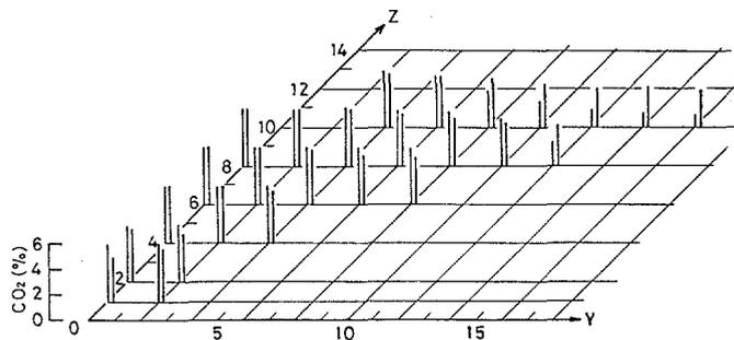
Fig.7 Spatial distributions of carbon dioxide in the upper half plane of the airgap when carbon dioxide is supplied at  $z=8.0$  mm. Gas flow is reflected upwardly by the magnetic fields.
