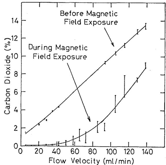
Fig.8 Concentration of carbon dioxide v.s. flow velocity. Flow of carbon dioxide is blocked or modified during magnetic field exposures. The airgap is 5 mm wide, and the field intensity is 1.36 T at the center of the airgap.
